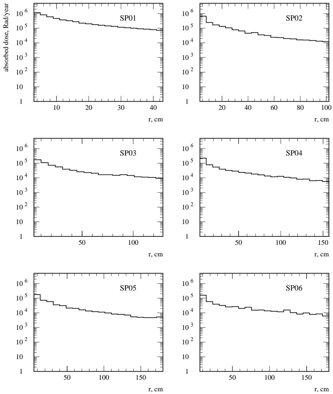
Figure 2: Absorbed dose level, Rad/year, as a function of distance from beam axis ( $r$ ), for silicon plates no.1–6.
