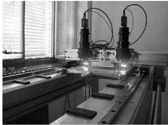
Figure 7 Laser soldering station (left); station for wire pitch and tension check (right).
