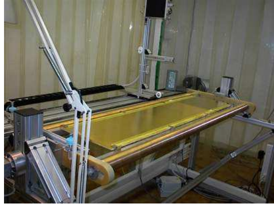
Figure 6 Gluing table for preparation of the panels (left); automated wiring machine (right). This machine can also be used for wire gluing.
