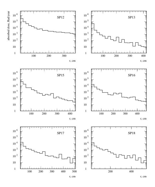
Figure 4: Absorbed dose level, Rad/year, as a function of distance from beam axis (r), for silicon plates no.12, 13 and 15–18.
