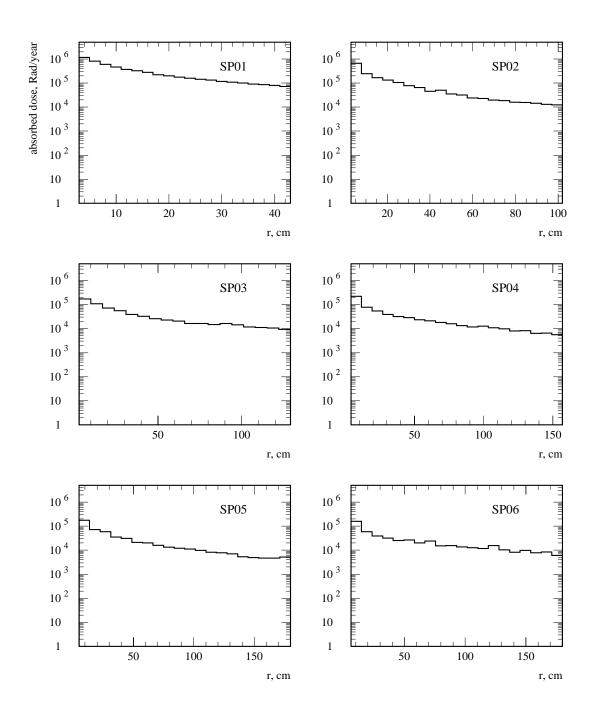
Figure 2: Absorbed dose level, Rad/year, as a function of distance from beam axis (r), for silicon plates no.1–6.
