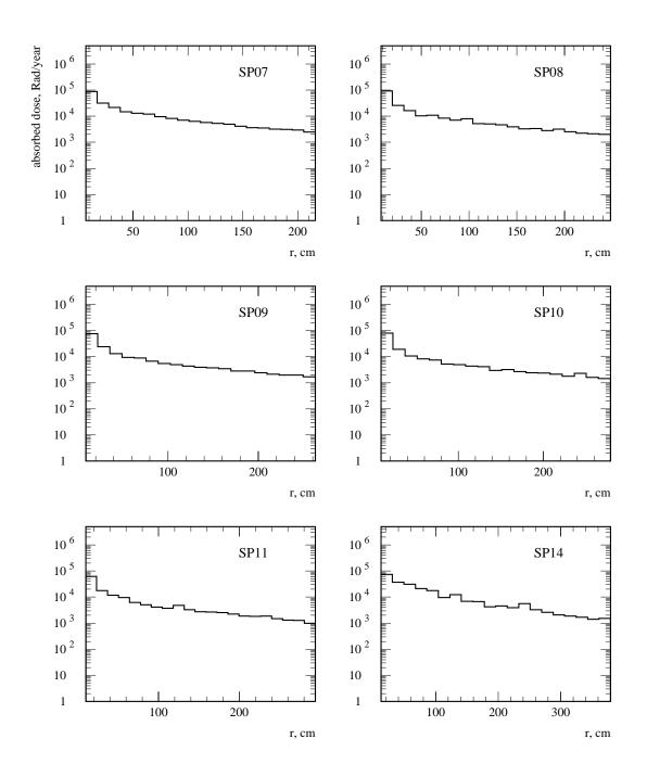
Figure 3: Absorbed dose level, Rad/year, as a function of distance from beam axis (r), for silicon plates no.7–11 and 14.
