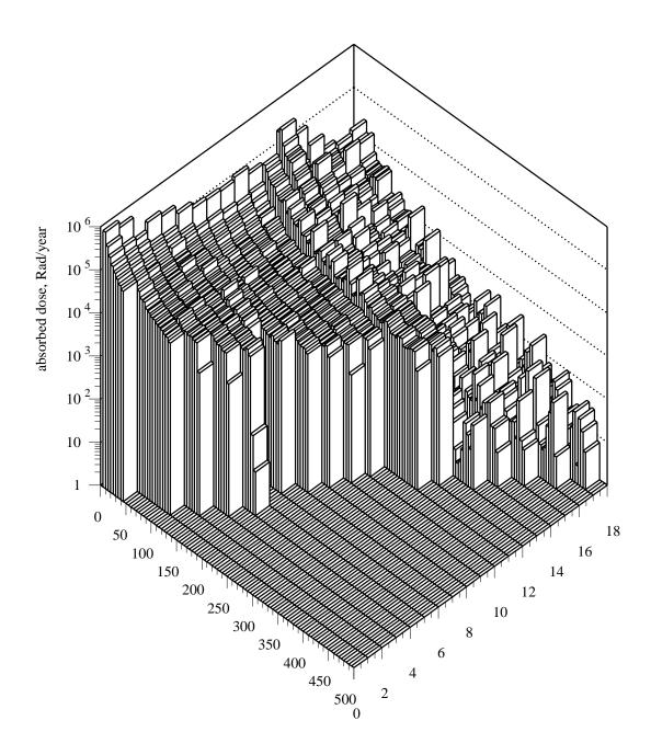
Figure 1: LHC-B absorbed dose level map, Rad/year, as a function of distance from beam axis (r, left axis) and silicon plate number (right axis).
