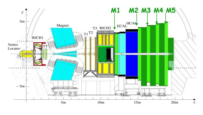
5 Muon stations M1 in front and M2-M5 behind the calorimeters
