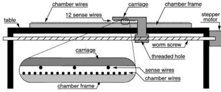
The wire is forced to oscillate by a periodic HV applied to a sense wire place parallel and close to it.
