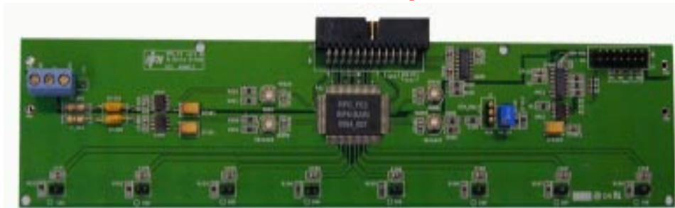
Prototype board used in beam tests (8 ch)
