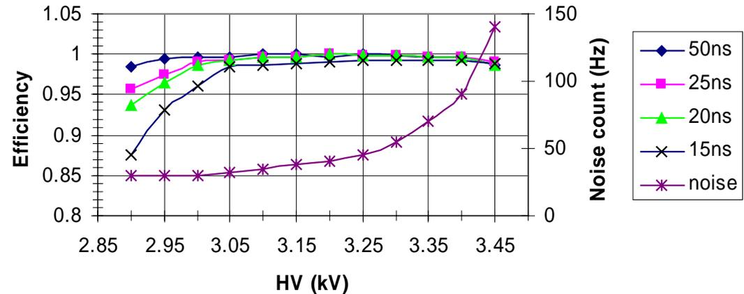
MWPC, cathode pad readout (Pad size 4x8cm)
