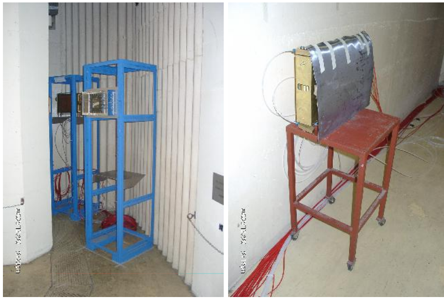
Figure 2: LEFT: The two racks supporting the MWPC test chamber (back) and the GEM (front) RIGHT: the monitor chamber mounted on a stool, placed behind a concrete wall.
