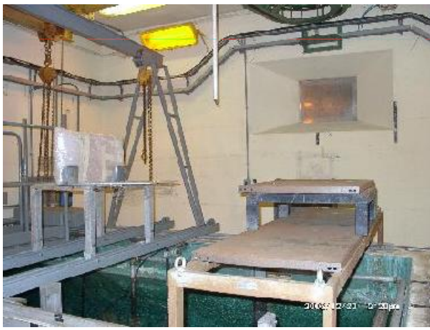
Figure 3: LEFT: The pool containing the source. RIGHT: the test chamber mounted on the rack at \sim 170 cm from the floor.
