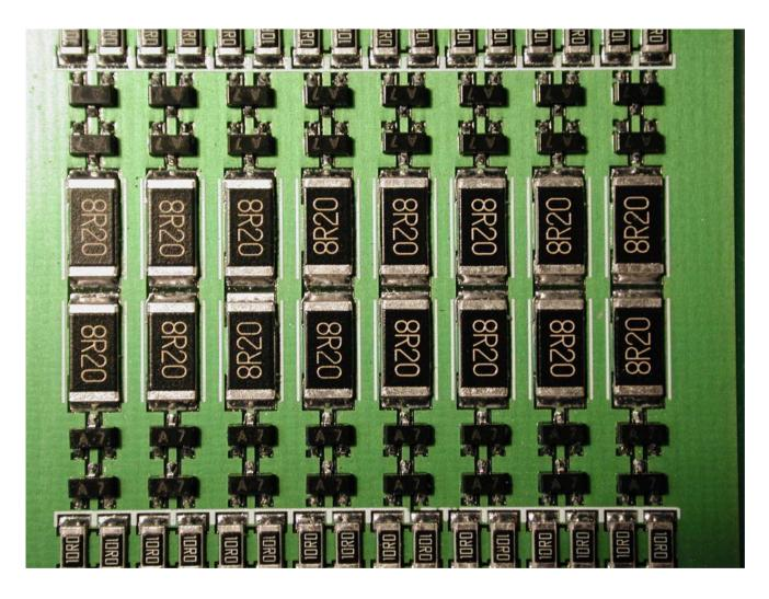
SPB no.5 - Card 63x20 mm2 – Wire readout - On the back LNF SPB3 ALL Dic 2003 SMD resistors are ~ 0.5 mm thick Logo of resistor not equal to spb no.3 All Frascati chambers have these !
