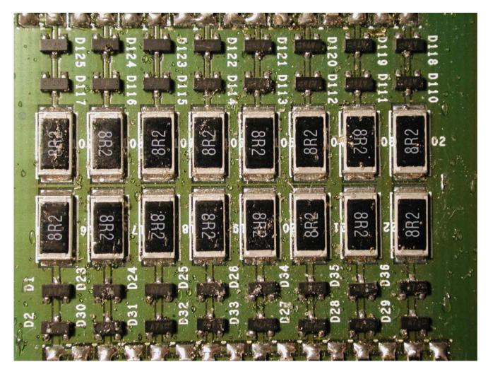
SPB no.1 - Card 70x20 mm2 - On the back INFN Roma1 2001 SMD resistors are ~ 1mm thick
