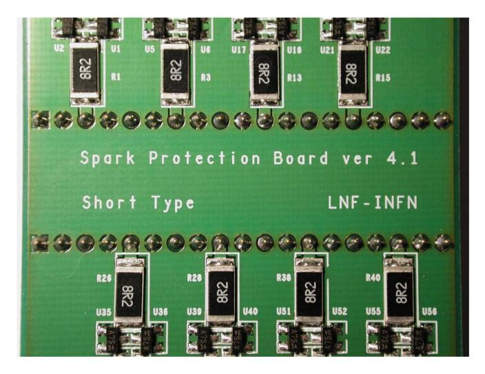
SPB no.6 - Card 63x20 mm2 – Pad readout SMD resistors are ~ 0.5 mm thick Only one found in Frascati Apparently same R type of spb no.3
