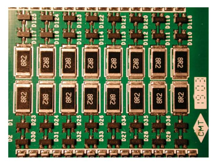
SPB no.3 - Card 70x20 mm2 - On the back LNF SPB3 NEW Apr 2002 SMD resistors are ~ 0.5 mm thick Apparently R is NOT equal to spb no.1 or 2
