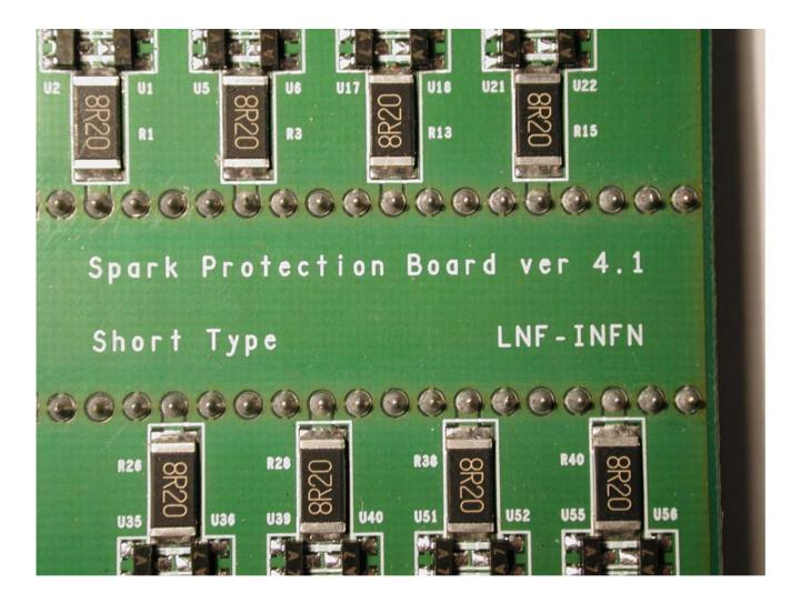
SPB no.7 - Card 63x20 mm2 – Pad readout SMD resistors are ~ 0.5 mm thick All Frascati chambers have these !
