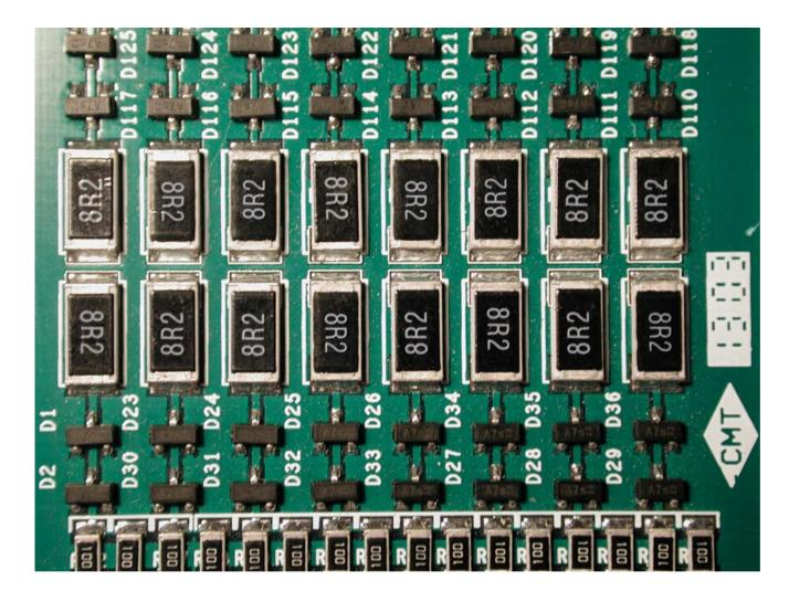
SPB no.2 - Card 70x20 mm2 - On the back LNF SPB3 NEW Apr 2002 SMD resistors are ~ 1mm thick Apparently R equal to spb no.1
