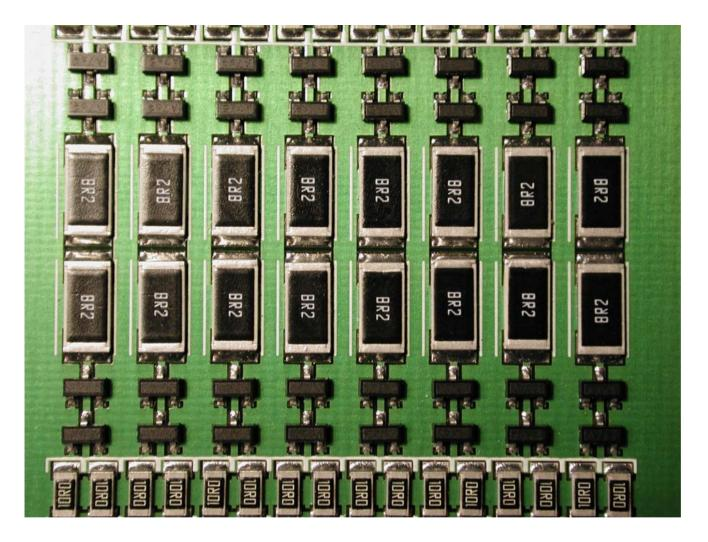
SPB no.4 - Card 63x20 mm2 – Wire readout - On the back LNF SPB3 ALL Dic 2003 SMD resistors are ~ 0.5 mm thick Logo of resistor not equal to spb no.3 Only one found in Frascati chambers (up to now)
