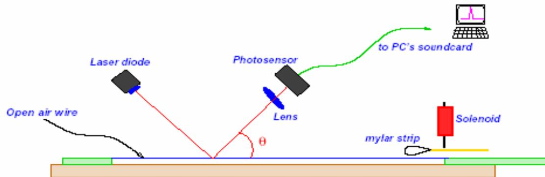
The wire, mechanically excited by a mylar hammer, vibrates with its own fundamental frequency; the light of a laser beam is reflected on the wire and then detected by a photodiode whose signal is sent to a standard PC sound card and then analyzed
