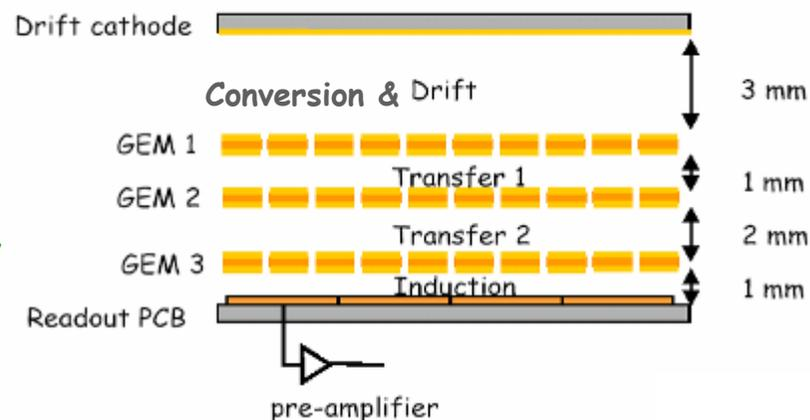
Rate Capability  $\sim 1 \text{ MHz/cm}^2 @ 5 \cdot 10^{32} \text{ cm}^{-2}\text{s}^{-1}$
