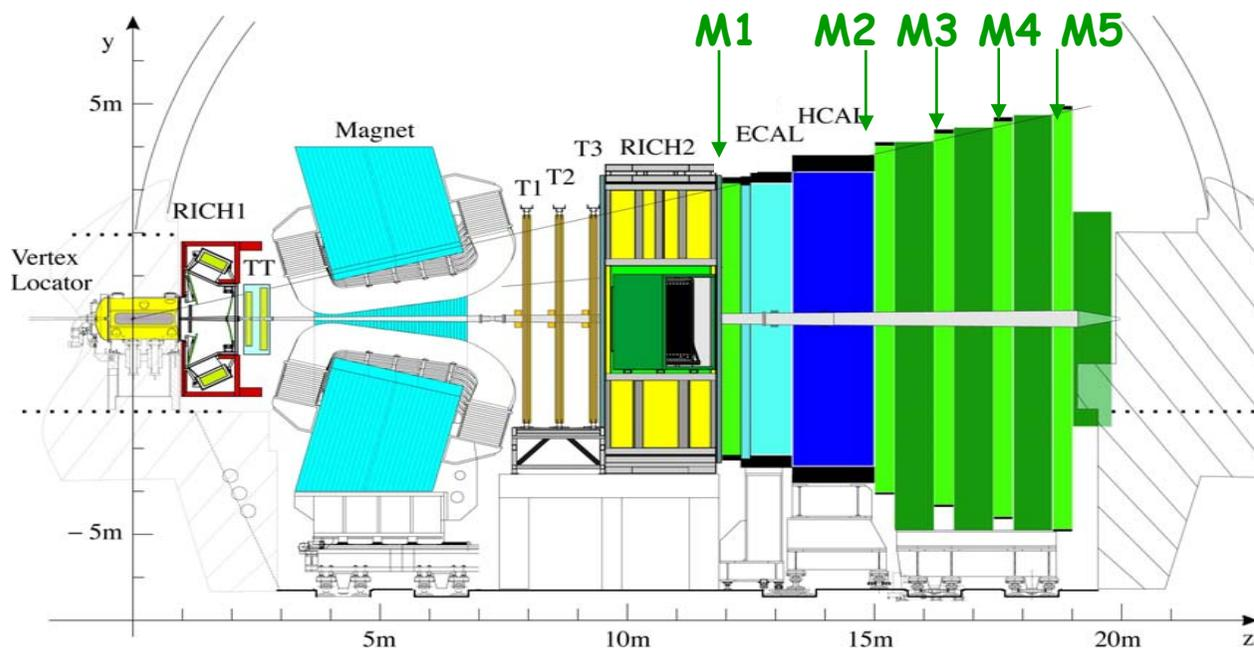
5 Muon stations M1 in front and M2-M5 behind the calorimeters
